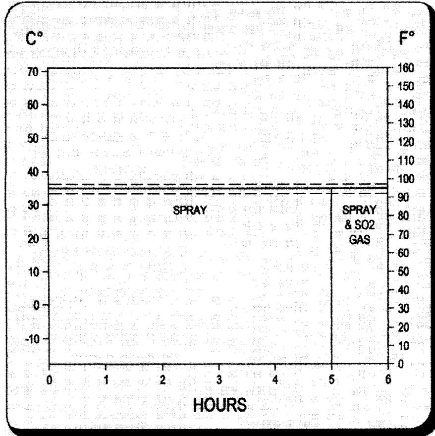
NOTE 1—Dashed chart lines indicate temperature tolerance limits.
