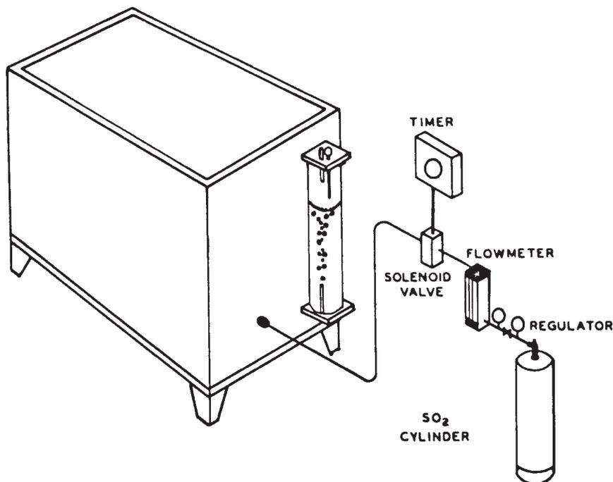
FIG. A4.1 Schematic of SO<sub>2</sub> Line into Salt Fog Cabinet
